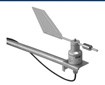
This highly professional wind direction sensor is manufactured for Adcon by one of Germanies's most reputed sensor manufacturers. The housing is made of extremely robust, seawater resistant anodized aluminum, to withstand even the harshest of conditions.
